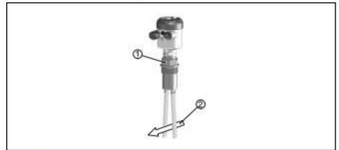
Fig. 7: Orientation of the tuning fork in case of flow
