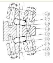
G1. Cover plate G2. Gauge glass G3. Mica gasket G6. Cushion gasket G7. Washer G8. Nut
