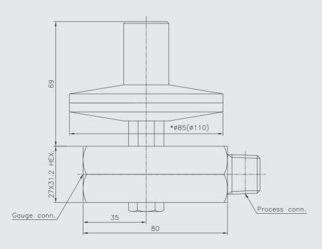
\*NOTE. Pressure 1~3kPa (Ø110), 3~50kPa (Ø85)
