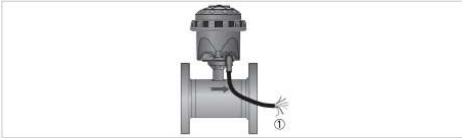
Figure 4-7: Output cable at IP68 compact version
